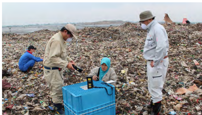
Fig. 3 Measurement of methane flux
